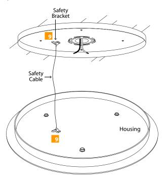
Insert one end of the safety cable into the mounting plate safety bracket and insert the other end into the housing safety bracket.
