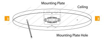
Align the mounting plate holes with the electrical box holes and mark four points onto the ceiling through the mounting holes.
